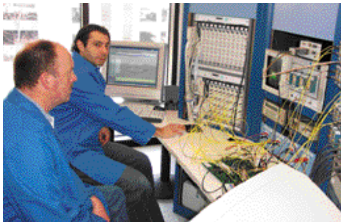
Sorin Grama and Marvin Kelly operate a station for testing mixed-signal devices. Courtesy of Cal-Bay systems and National Semiconductor.
